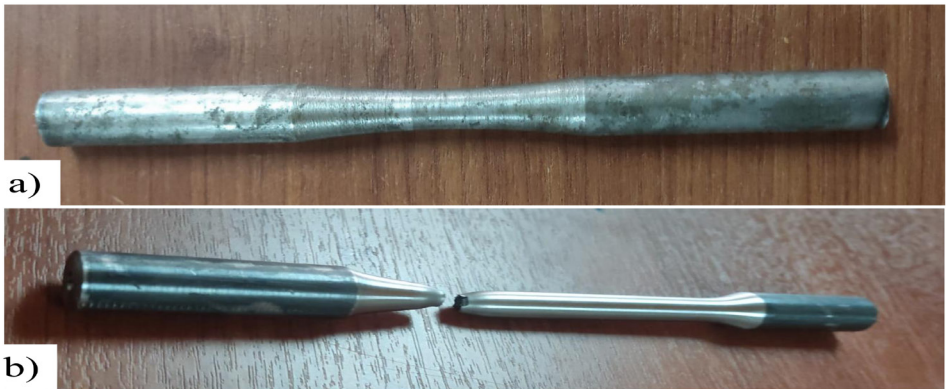
Figure 2 Specimen a) machined, b) after tensile test
